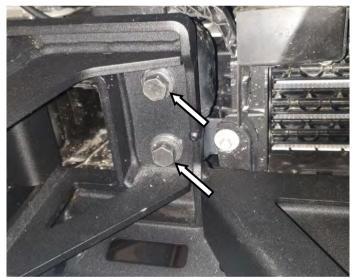
83. Using 3x M12x40 flange head bolts, hardened washers, and flange nuts, attach the bumper to the vehicle. Also install a M10x40mm flange head bolt, washer and flange nut to the drilled pinning hole. Leave finger tight for now.
