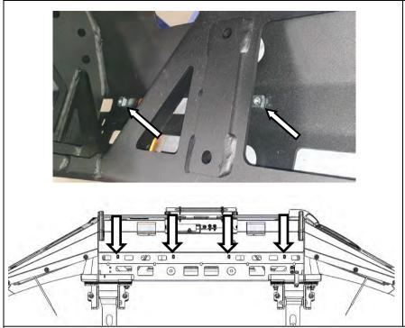
38. Install 4x M6 cage nuts into the bottom of the bull bar.
