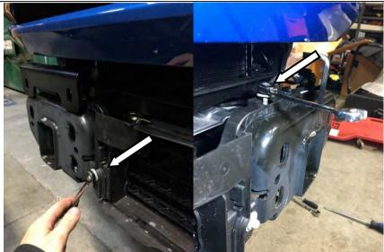
12. Remove the 4x bolts holding the intercooler shutters onto the vehicle. Remove the connector and clips to get the harness off the shutters.
