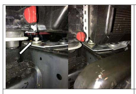
30. Loosen the top intercooler mount plate.
