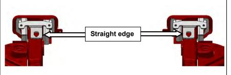
31. Chassis mounts are to be assembled as shown. The LHS brackets have identifier holes on them as the brackets are not symmetrical from side to side.
