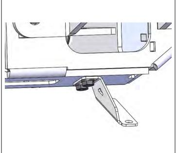
79. Install lower pan brackets using 2x M6x20 bolts, flange nuts, and washers.
