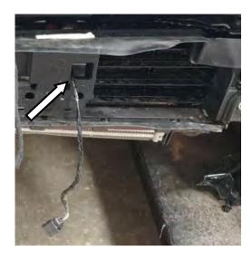
14. Fit intercooler shutter back in place with the extended camera loom routed as shown.
