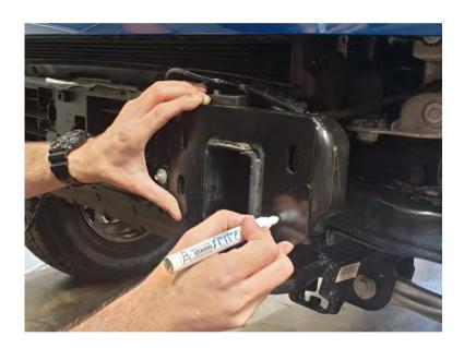
35. Using one of the 2mm chassis packers as a template, mark the pinning hole on both chassis end plates as shown.
