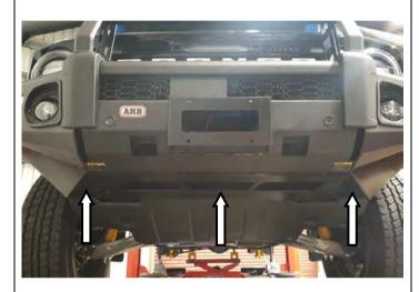
107. Fit self tapping pan head screws through the under panels into the OE plastic panel in the 3 places shown.
