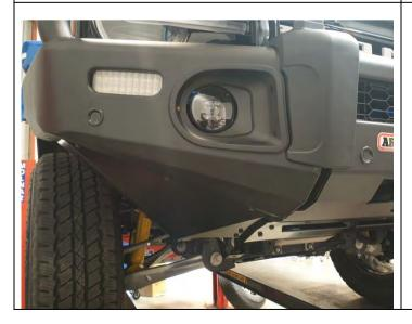
105. Install the wing under panels as shown using 6x M6x20mm bolts, washers and flange nuts.
