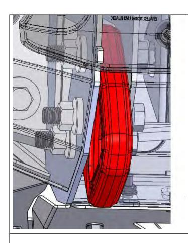
78. Insert recovery points in the orientation shown below and attach using 3x M12x60 flange head bolts, hardened washers, and flange nuts.
