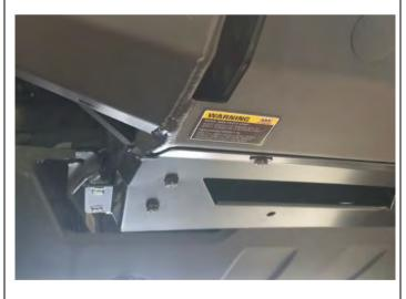
108. Fit Recovery point warning label on each side just below the recovery point aperture as shown.
