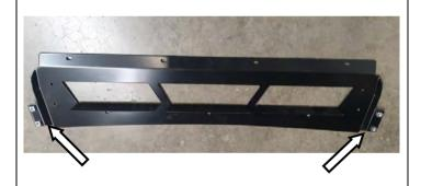
100. Fit 4x M6 cage nuts to the stone shield as shown.
