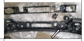
Remove factory nut plates by loosening plastic nut on back of the chassis end plate.
