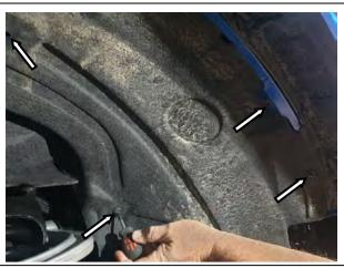
23. Remove the 4x screws and clips holding the wheel liners in place.
