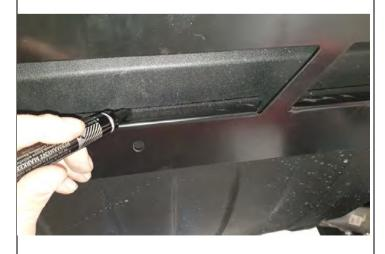
101. Hold the stone shield in place and mark the plastic OE panel where the stone shield clashes with it.
