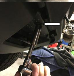
3. Remove 6x bolts holding the under tray on and retain for refitting the under panel later.
