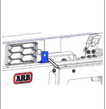
59. Using an M6x20 bolt, flange nut, and washer, attach the grille bracket into the centre locations as shown.
