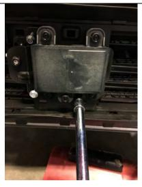
Remove factory radar cover and radar (if optioned) by removing the 3x screws under the cover. Set the radar aside as it will be re-used. Discard the radar cover.
