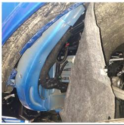
24. Peel back wheel liners to gain access to the rear of the headlight.
