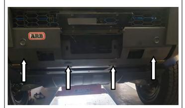
106. Fit 35mm plastic caps to the 4x holes as shown.
