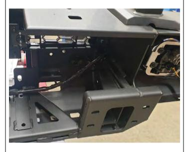
81. Using harness removed from the stock bumper, route it through the new bumper to the parking sensor housings (if installed) and foglights.
