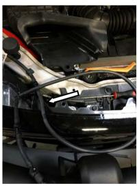
22. Both the wiring and washer fluid line will need to be routed to the front of the Summit bar. Trace both back to the headlight area and then reroute under the fascia.
