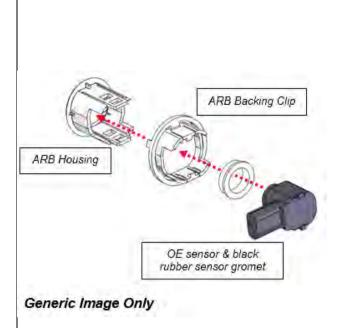
80. Install 2x **outer** parking sensor housings into the wings of the bumper if parking sensors are optioned. Otherwise, install blanking plugs.
