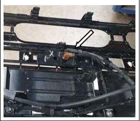
21. Using the 500mm of washer fluid line, extend the existing line to allow it to reach the relocated camera.
