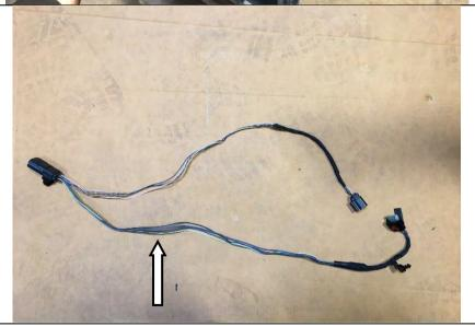
13. Using a razor, carefully strip back the loom all the way to the connector to allow for more movement in the harness. Tape the exposed wires back up with black electrical tape or cover with flexible conduit.
