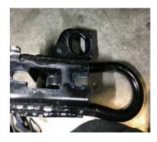
10. Remove bolts holding on factory tie down points and set aside. If these have the integrated intercooler mounts, they will be re-used.
