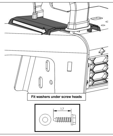
66. By aligning the front buffer with the tongue of the rear buffer, attach the front buffers to the front face of the bar. Ensure each buffer sits flat against the face of bar and is keyed into the top section of the rear buffer.
