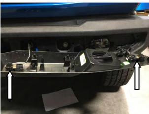
2. Unclip the parking sensors from the housings but leave them connected to the loom.
