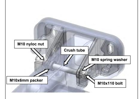
34. Using the 2x M10x110mm bolts, 6mm packers, M10 spring washers, nyloc nut and crush tube, assemble the lower bolt for the chassis brackets as shown.
