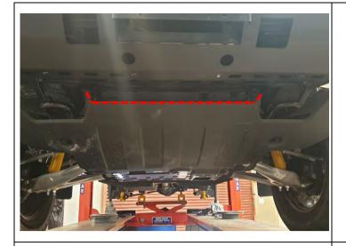
102. Trim the plastic OE panel as shown using an oscilatting multitool or jig saw.
