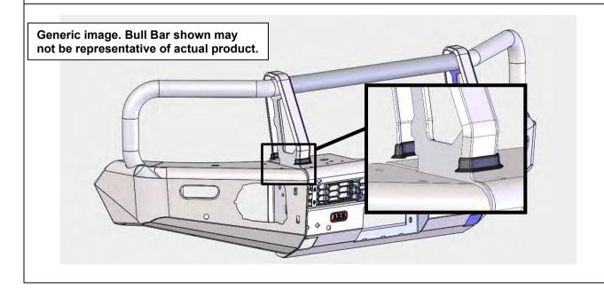
65. From the rear of the bar, slide the rear buffer sections under the rubber mouldings.
