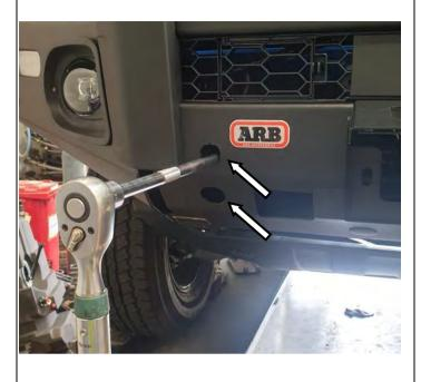
93. Tighten the 3x M12 and 1x M10 chassis mount bolts per side to the specified torque. Access to the inboard bolts can be made through the parking sensor holes and lower holes in the lower pan as shown.
