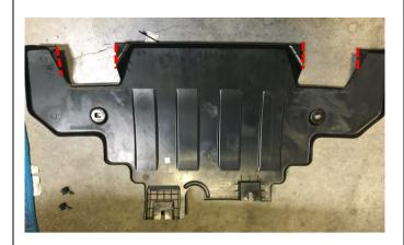
97. If your vehicle has a plastic stone guard with OE tow points, the area surrounding the tow points needs to be trimmed out as shown using an oscilatting multitool or jig saw.
