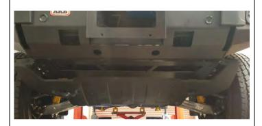
103. Install the stone shield as shown using 8x M6x20mm bolts, washers and flange nuts.
