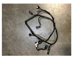
8. Remove the wiring harness for the parking sensors and fog lights and set aside for fitment into the ARB bar.
