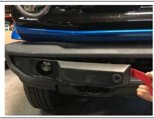
Remove plastic panels covering the bolts on the front bumper. (On some models these will also include the parking sensors).
